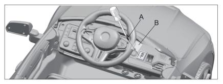
A.Remove the screw on the protective cover (on the dashboard) with a screwdriver.
